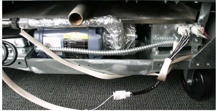
Figure 5: Attach the provided harness to the 9-pin plug on the transformer box in the pin locations occupied by the existing heater tape wiring ( pins 1 and 3) and connect the existing and the new heater pate to the 4-pin plug on the harness shown partially wired above.
