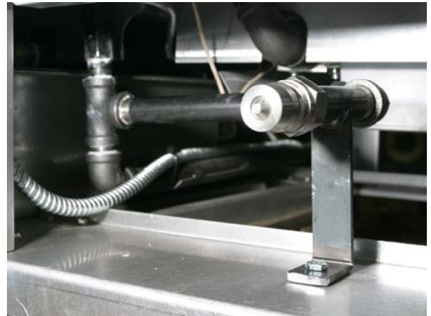
Figure 2: Position the T in the return line and attach the quick-disconnect and its related hardware as shown. Drill a hole in the fryer channel to secure the bracket with a 1/4x20 machine bolt and nut.
