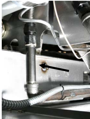
Figure 1: Remove existing pipe above the elbow (see arrow) for insertion of a T provided in the kit.
